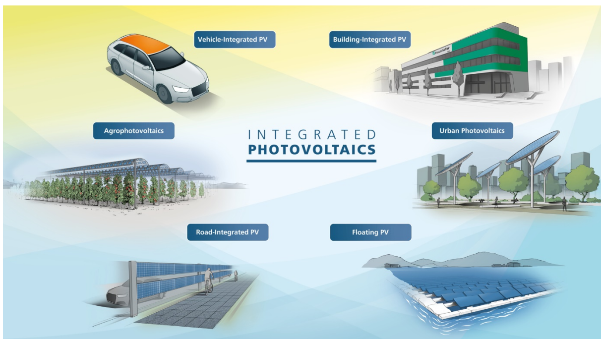
Figure 29: Applications for the integration of photovoltaic
